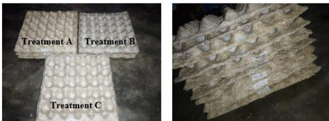
Figure 2. Fabricated bio-composite egg trays.
